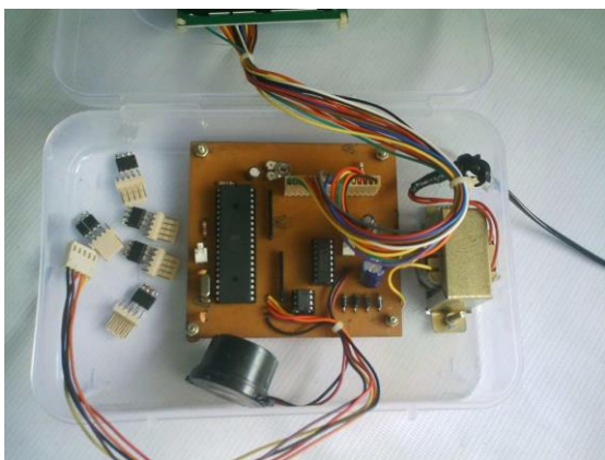
Fig. 2. Actual designed model of prepaid energy meter.
