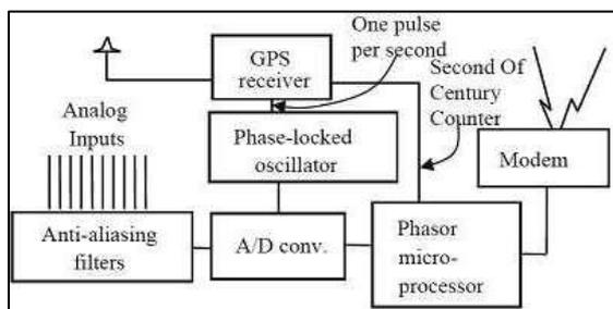
**Fig. 1. Functional Block Diagram of PMU.**
