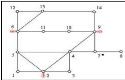
Fig. 2. IEEE-14 Bus System With PMU Placement.
