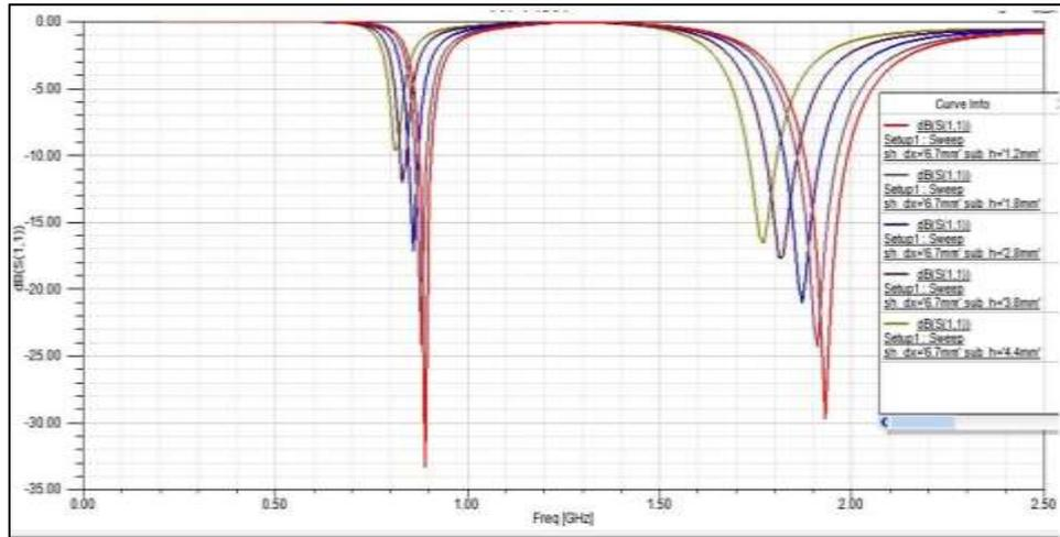
Fig.10: Return Loss Corresponding To Substrate Height Variation.
