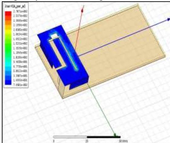
**Fig 15 (a):** Surface Current Distribution at 0.89GHz.
