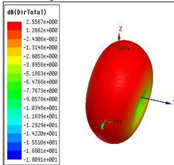
Fig. 13: Directivity Plot for  $f_r = 0.89\text{ GHz}$ .
