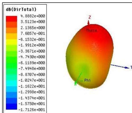
Fig. 14: Directivity Plot for  $f_r = 1.93\text{ GHz}$ .
