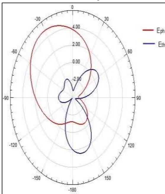
Fig. 12: Radiation Pattern for  $f_r = 1.93\text{GHz}$ .
