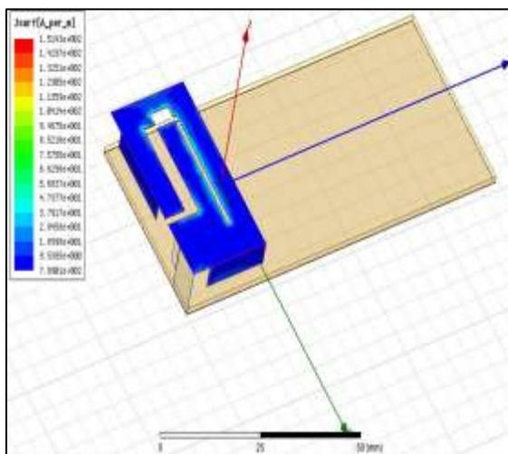
**Fig 15 (b):** Surface Current Distribution at 1.93GHz.
