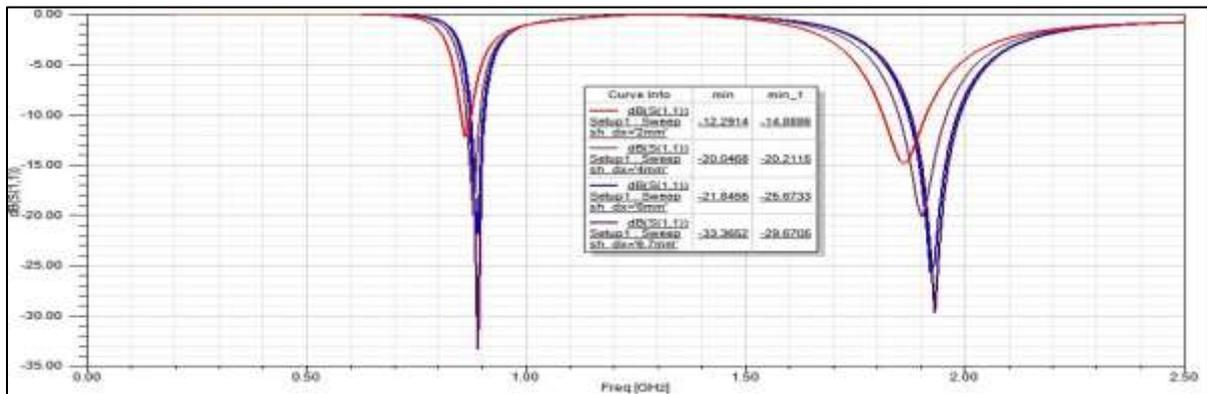
Fig. 9: Variation of Return Loss with Frequency for Different Short Plane Width.
