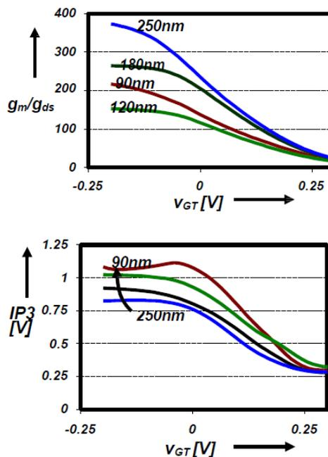
**Fig. 1:** Various DC-Properties of Transistors as a Function of the Gate-Overdrive Voltage with  $V_{DS} = 0.3$  V and  $L = 1$   $\mu$ m for Four Technologies: (a) the Gain, and (b) the Output IP3.
