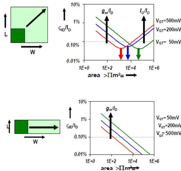
**Fig. 3:** The Spread of an MOS Transistor in 65 nm CMOS with (a) Linear Scaling of W and L at Constant Power Consumption, (b) W-Scaling, and Proportional Power Scaling.
