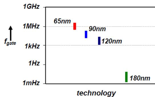
**Fig. 2:**  $f_{gate}$  Ranges for Typical Analog Applications, for NMOS-Transistors in Different CMOS Technologies. For PMOS-Transistors  $f_{gate}$  is roughly a Factor 3 Lower.
