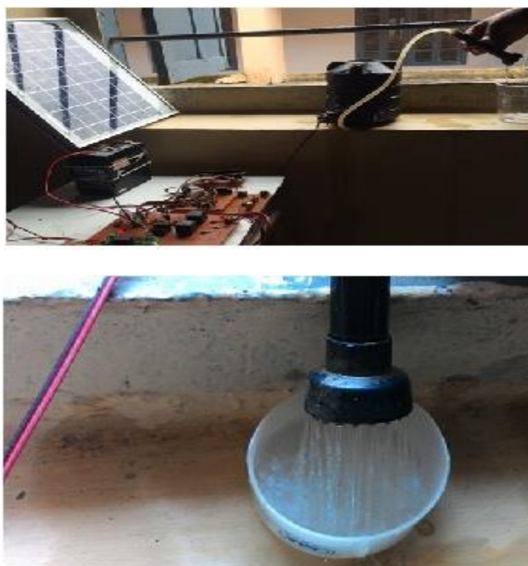
Fig. 23: Prototype Model of Water Pumping.
